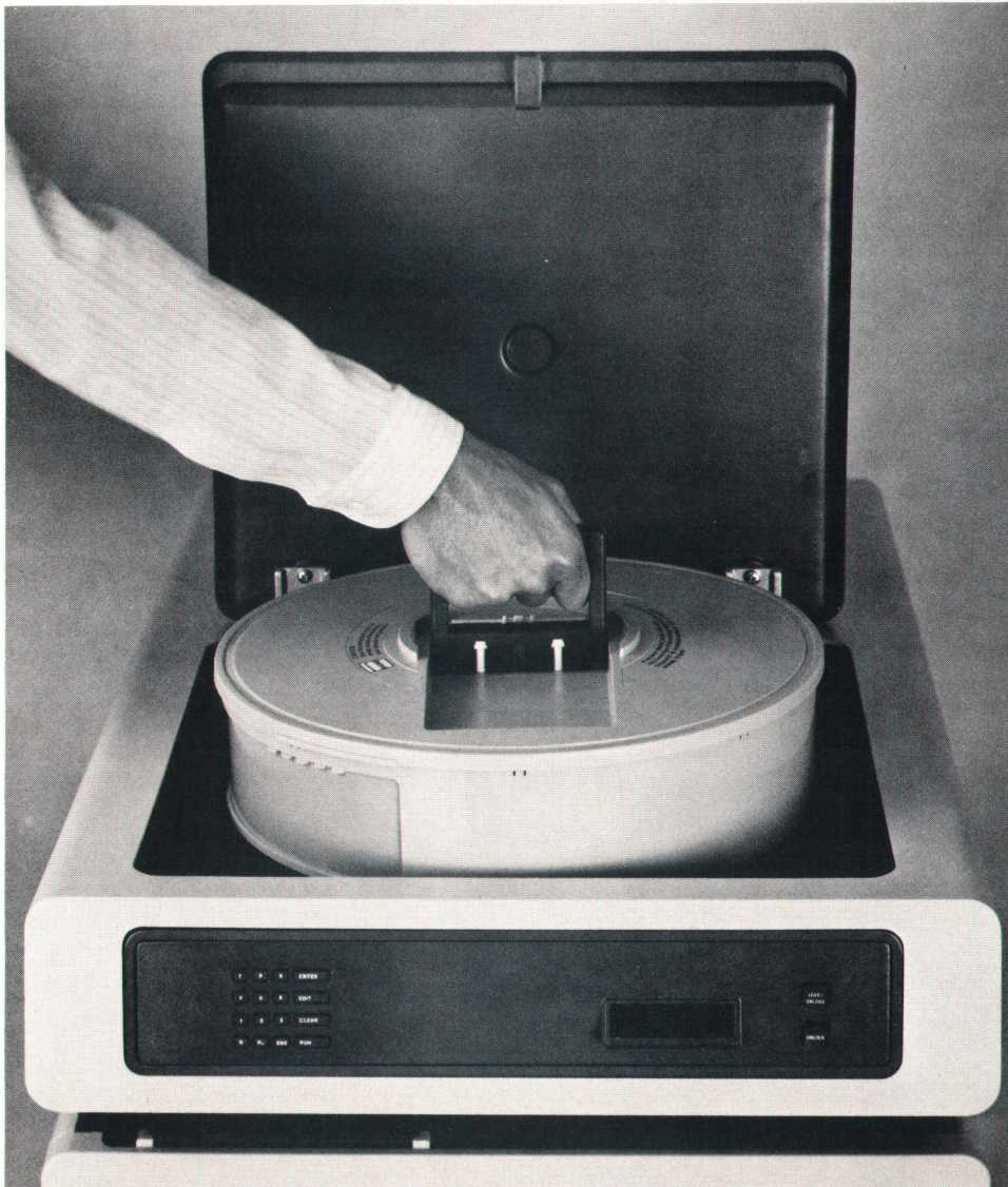
Fig. 2. The HP 97935A Data Pack for the 7935 Disc Drive provides contamination resistance similar to a sealed chamber. When the pack is inserted in the filtered air of the drive, a trap door opens to allow the heads access to the media.
